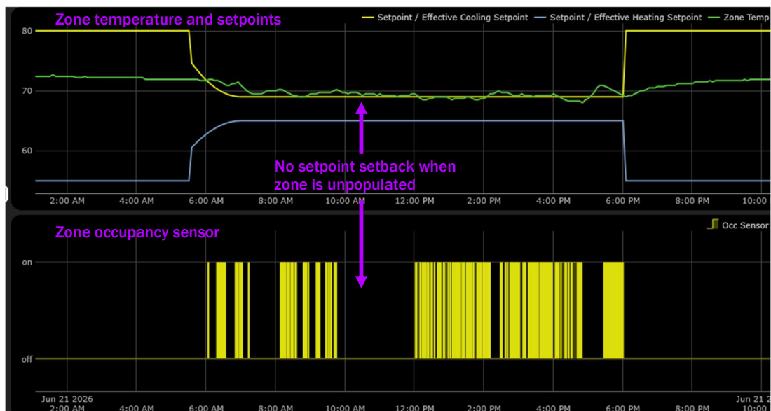
Figure 7: Indication of missing occupied standby.
