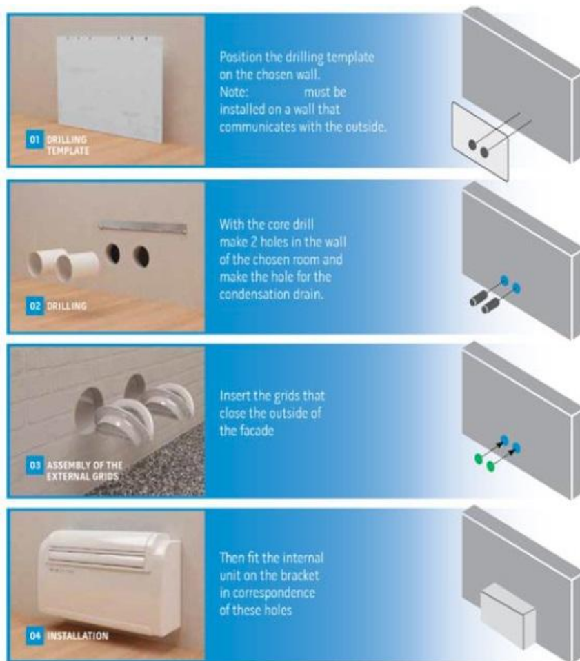
Figure 7: DDPHP installation process.
