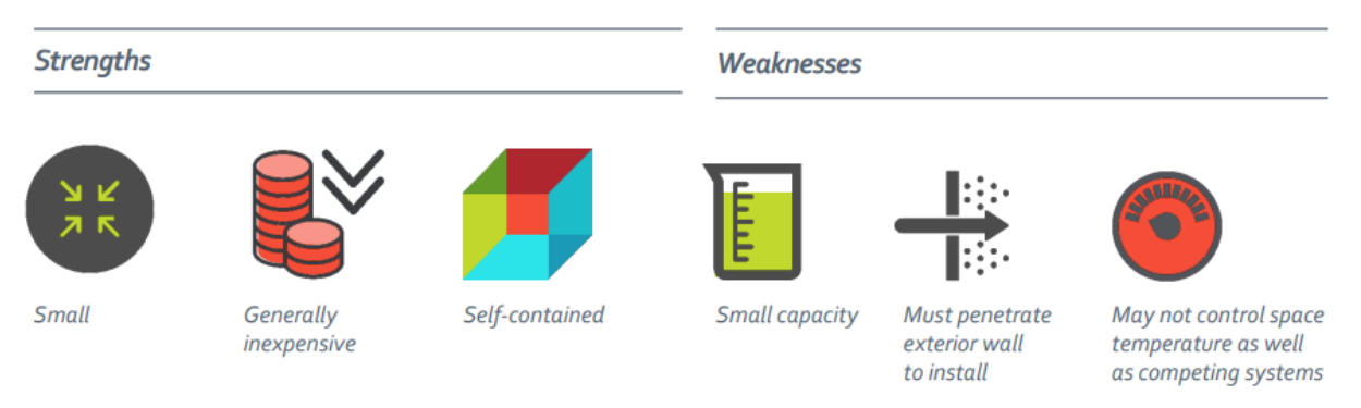
Figure 3: PTHP and PTAC design strengths and weaknesses.
