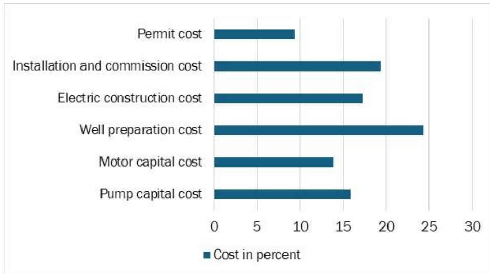
Figure 27: Customer pump installation cost estimation.
