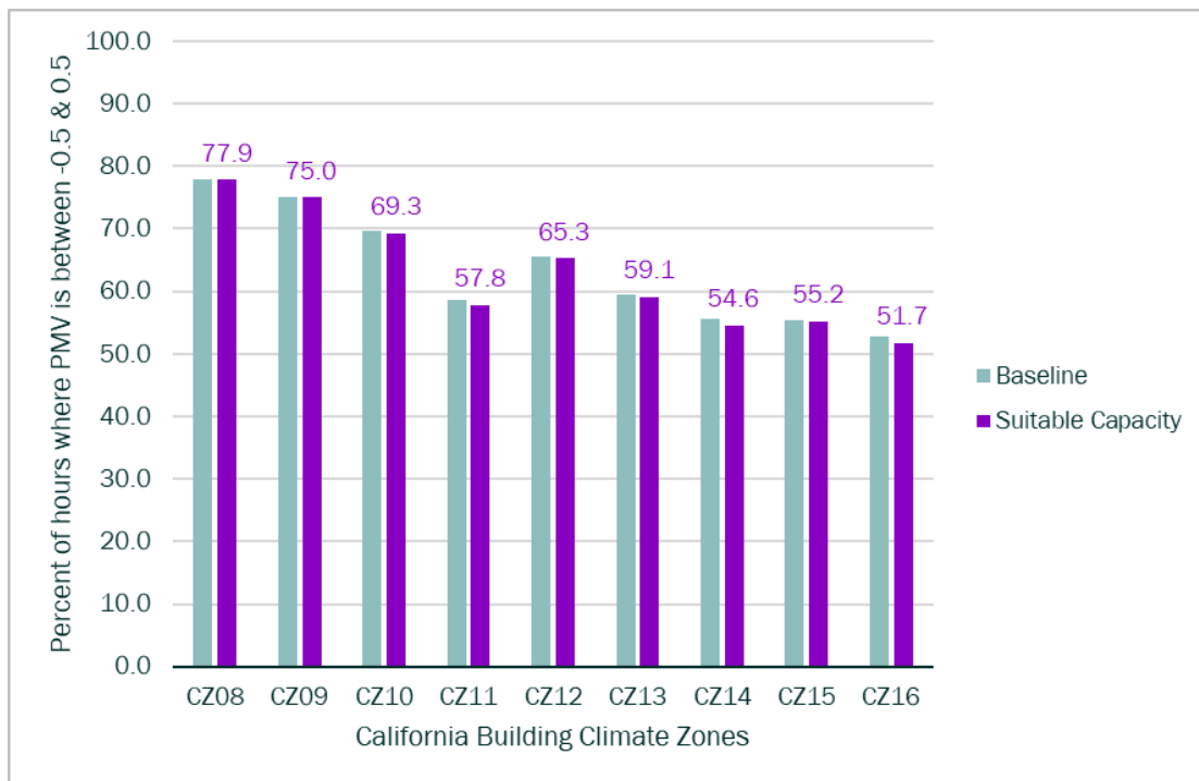
Figure 44: Percent of hours where PMV is between -0.5 and 0.5 in a pre-1978 MF upper corner unit living room facing South with door open and a ductless suitable capacity ASHP configuration.
