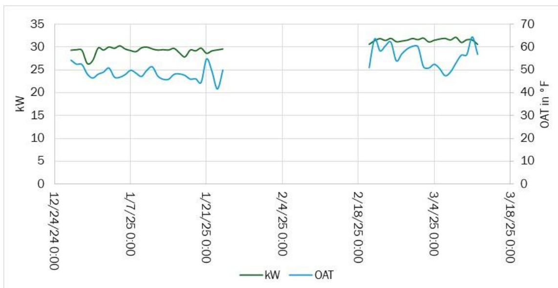
Figure 33: Westside chiller system kW profile.
