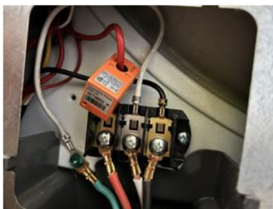
The Wi-Fi current sensor
