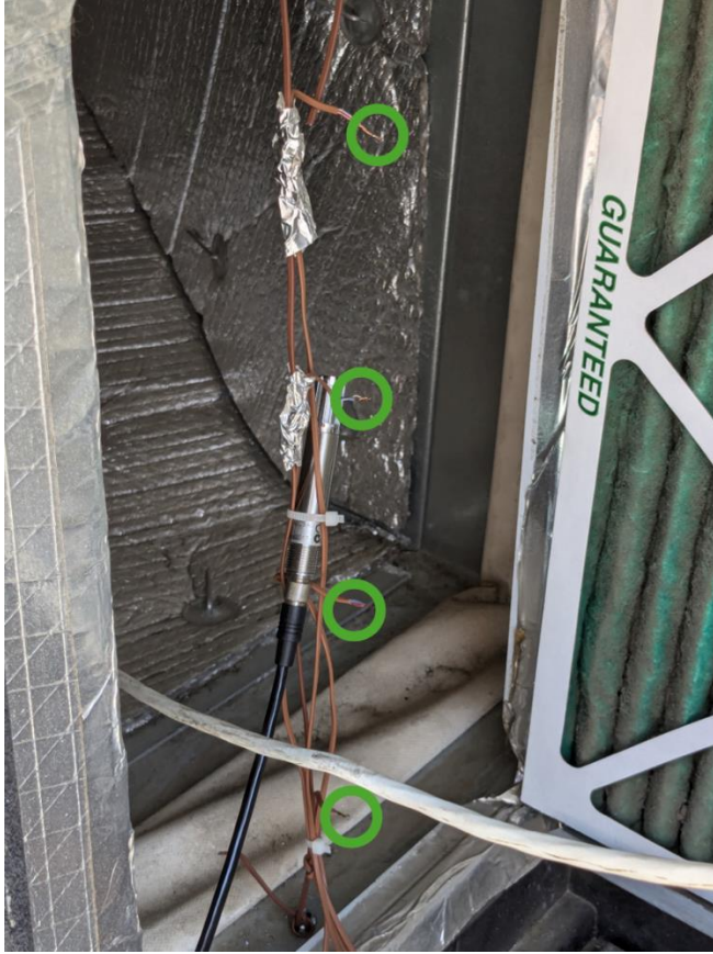
Figure 3. Thermocouples array and temperature humidity probe installed on return of gas-fired RTU
