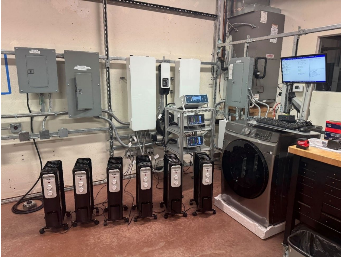
Figure 6: Smart panels lab setup, including test loads, measurement and verification system, and panel infrastructure.
