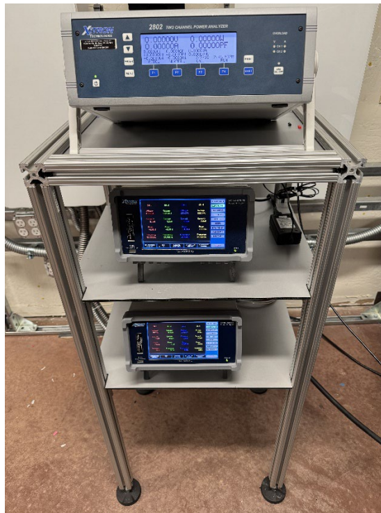
Figure 4: Metering equipment- Xitron 2802 (top) and the two Xitron XT2640AH (bottom)
