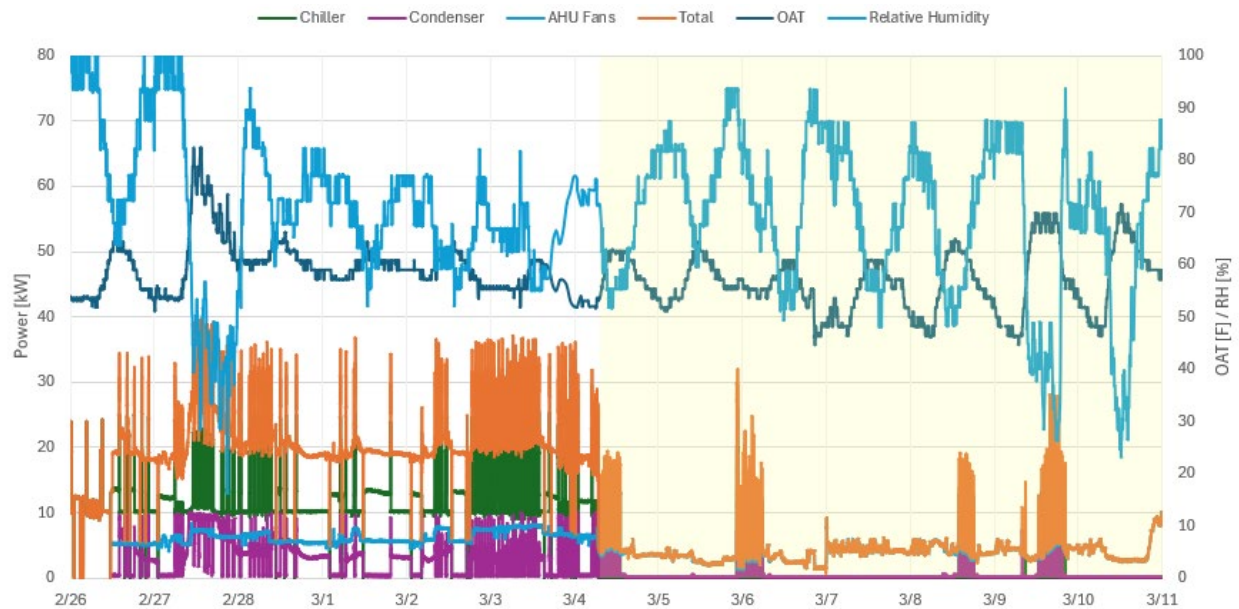
Figure 21: The operational profiles of chiller, condenser, and AHU fans during the two-week winter testing period in February and March.
