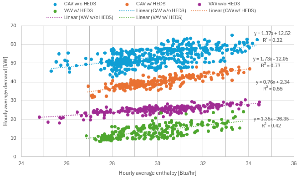
Figure 16: Hourly average total system power demand plotted against hourly average enthalpy of ambient air at four different test scenarios.
