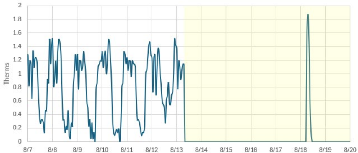
Figure 13: Gas consumption of HHW boiler during the two-week summer testing period in August.
