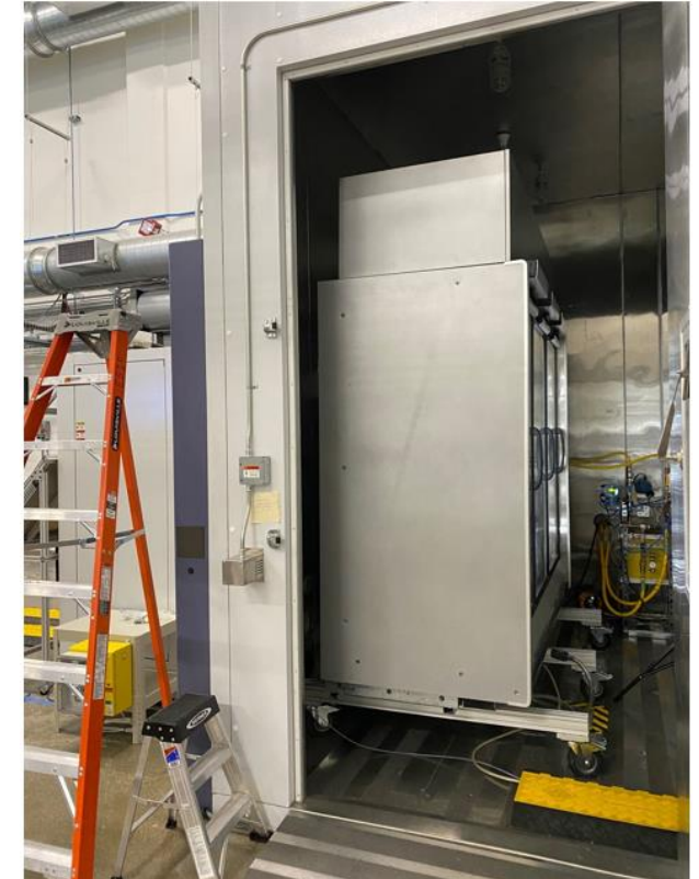
High efficiency water-cooled, low-GWP refrigerated display case inside the environmental chamber at NREL
