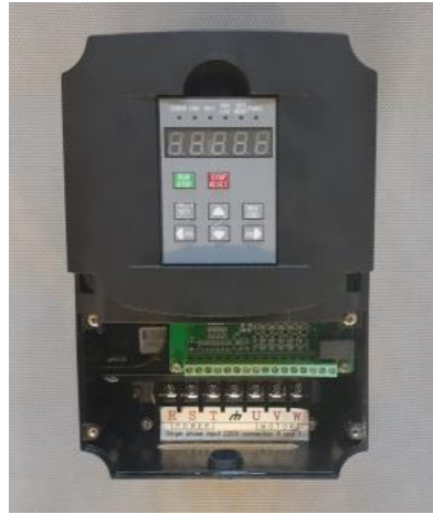
Figure 2: VFD internal wiring.
