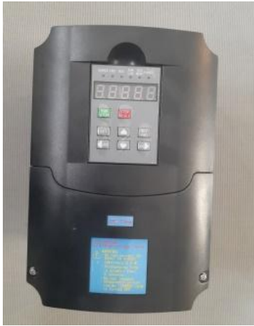
Figure 1: Variable frequency drive (VFD).
