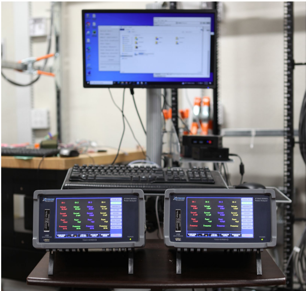
Figure 2: Metering Equipment: Xitron XT2640AH (left) and the Xitron XT2640AX (right). Data acquisition terminal (PC) in the rear of the two meters.
