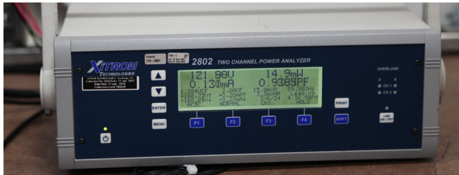
Figure 3: Xitron 2802 used for inline measurement.
