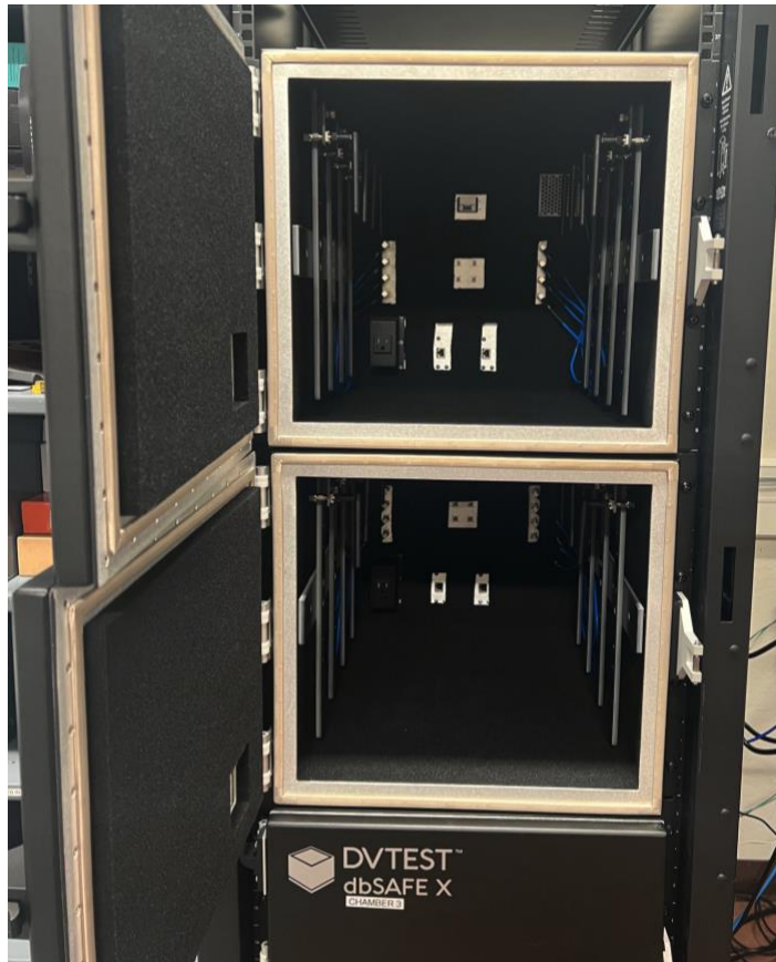
Figure 4: Anechoic chamber with attenuation antennas mounted
