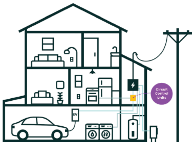
Figure 6: Circuit control units.
