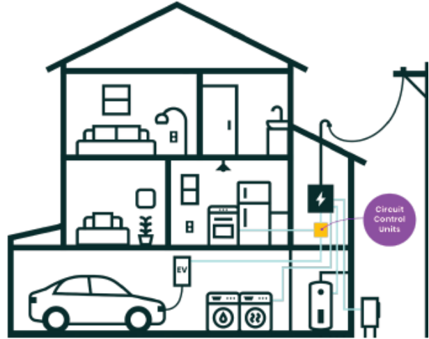
Figure 2: Circuit control units.
